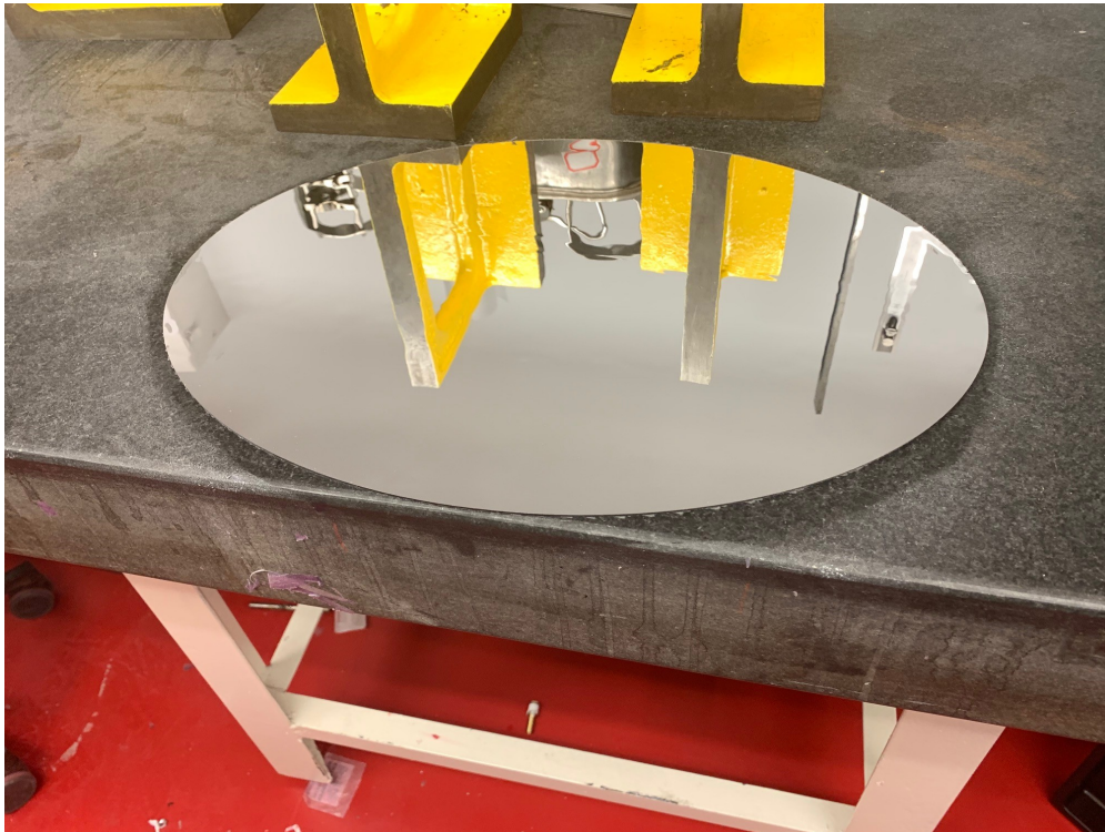
Figure 3: The Lexan and carbon fiber assembled mirror, before installation into the Cherenkov tank.
