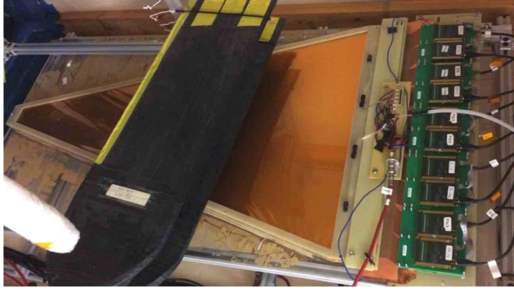
Figure 12: EIC GEM prototype-II built by the UVa group (pictured here installed and tested in the UVa X-ray test facility with APV-25 electronics). This GEM module will be used for the VMM and APV-25 readout evaluations proposed in the DAQ part of the pre R&D plan presented here. The main features of this prototype: geometry, size, the readout structure and the read-out strip layout (with all channels being readout from the other edge of the module), are all similar to what is proposed for MOLLER GEMs. As such, this prototype provides an excellent test-bed for the evaluation and benchmarking of the readout proposed here.
