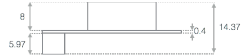
Figure 3: Side view of the FEASTMP module with mechanical dimensions.
