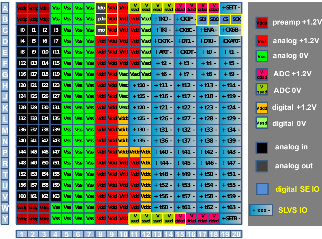
Figure 7: VMM3a pinout (top view)
